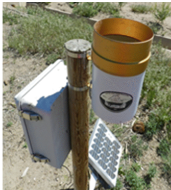
Figure 4 Standard (A) data logging (B) rain gauges and dirt and residues accumulated on a data logging rain gauge in which periodical maintenance has not been undertaken adequately (C)
