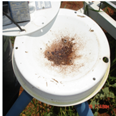
Figure 4 Standard (A) data logging (B) rain gauges and dirt and residues accumulated on a data logging rain gauge in which periodical maintenance has not been undertaken adequately (C)
