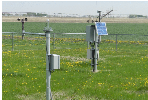
Figure 2 Basic weather station with the minimum sensors needed for the estimation of the reference evapotranspiration
