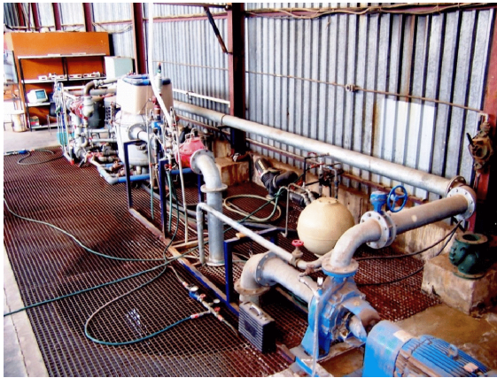
Figure 12 The fully automated filter test bench in the Hydrolab of ILI
