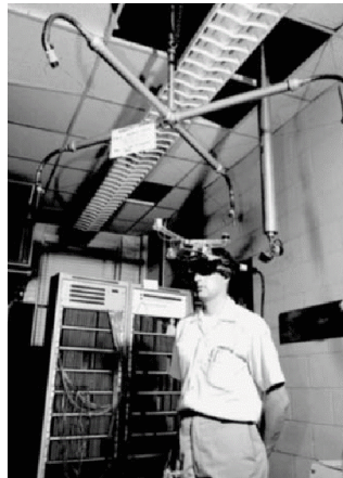
Figure 2 Head-mounted display by Sutherland (1968)
