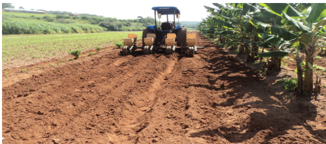
Figure 13 Experimental mechanized seeding and furrowing
