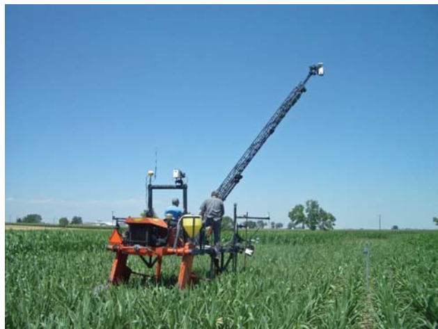
Figure 3. High Boy reflectance tractor measuring canopy ground cover, reflectance and temperature
